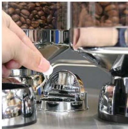
9. Lift dome lid and drop in one Schaefer cleaning tablet. Close lid after dropping tablet. **Note:** Dome lid is located behind front center hopper for 3 grinder machine configuration.
